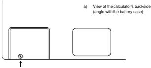
Screw for opening the battery case
