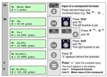
The bracket function is not disposable in the calculator mode. It can only be used for the input of compound formulas in the stoichiometric menus.
