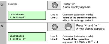
**Remark:** Multiplication and other operations of the atomic mass unit with constants of function "C" can only be performed after memorizing the first value in one of 10 memory places (see ch. 9.2.2 p. 79).
